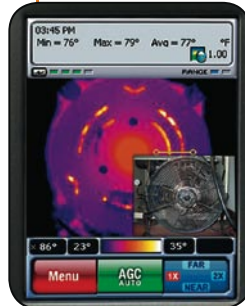
▲ Visible camera output shown in picture-in-picture mode (1 of 4 modes available)
